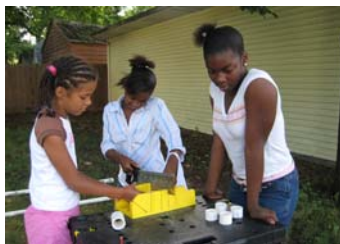
Summer youth participants learning how to accurately measure with a tape measure, use a miter box, and hand saw to cut pieces of PVC piping to make a carnival game.
